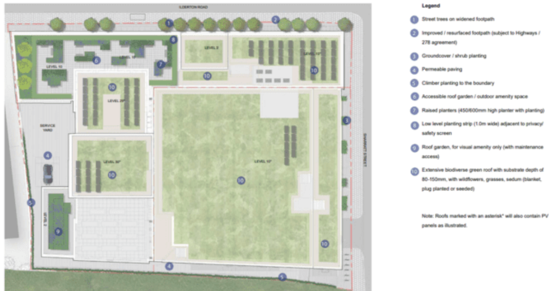
Image 34 (above): Roof plan showing the landscaping arrangement
