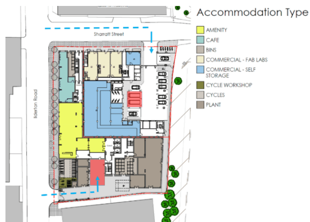
Image 36 (above): Routing strategy for servicing the proposed development with the servicing facilities highlighted in red and the routes in blue
