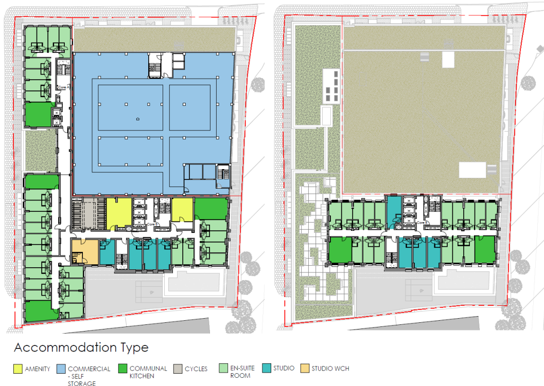
Image 16: Left: Typical layout of the shoulder block (2/F – 9/F), showing the dual aspect nature of the communal kitchen/living/dining spaces of the cluster flats in the Core A (West Core). Right: Typical layout of the tower block (12/F – 18/F), showing the dual aspect nature of the communal kitchen/living/dining spaces of the cluster flats
