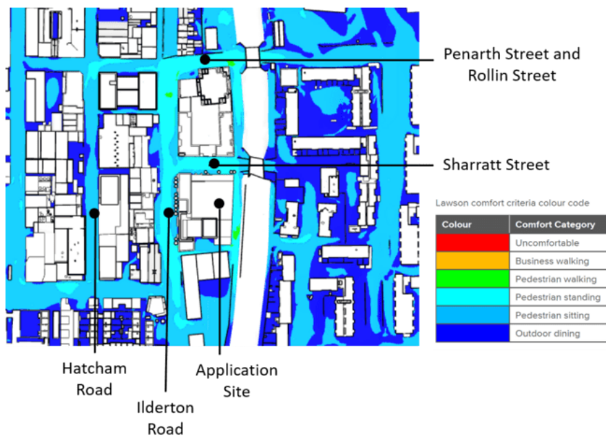
Image 38: Pedestrian wind conditions at ground plane in the proposed development, with mitigation, within cumulative surrounds
