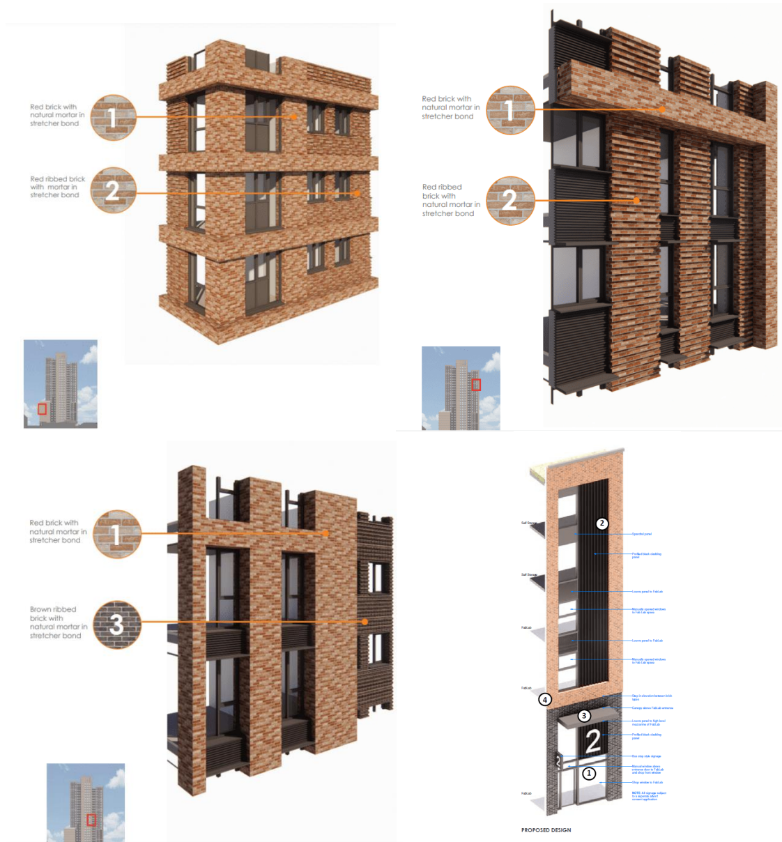
Image 26 (above): Typical elevation of the buildings. (a) shoulder block of the PBSA (top-left), (b) the wings of the tower block (top-right) ; (c) central section of tower block (bottom-left); (4) Fab Labs (bottom-right)
